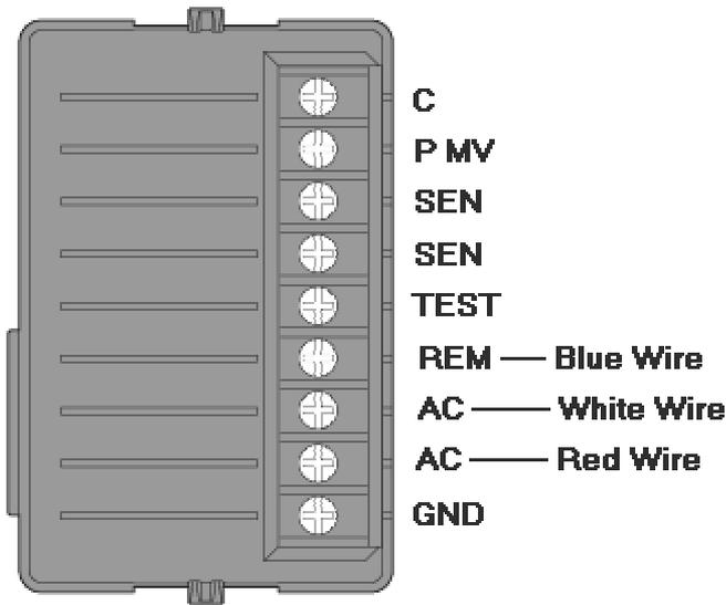
The Blue wire is connected to the terminal marked “REM”
