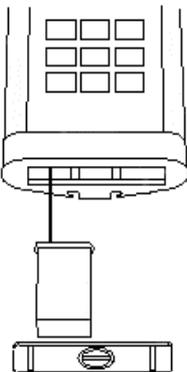
Remove the battery door (cover) on the underside of the transmitter to replace the battery
