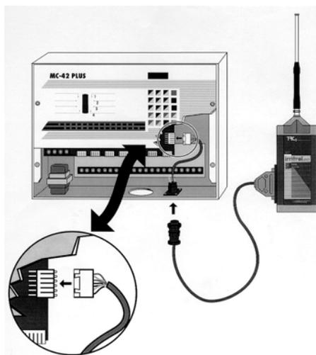
**NOTE: ALWAYS CONNECT THE DCI-2 TO THE RECEIVER FIRST OTHERWISE THE RECEIVER WILL BE DAMAGED INTERNALLY AND NEED TO BE REPAIRED.**
