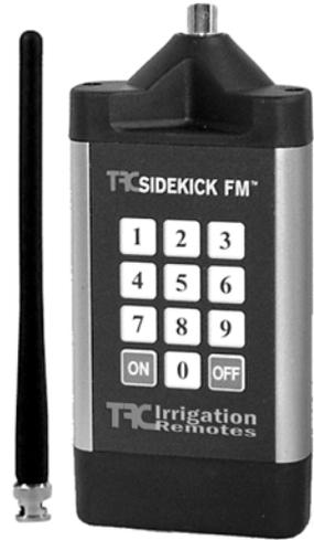
When not in use the transmitter reverts to a standby mode, which is designed for minimal power consumption to extend the life of the battery. Once any key has been pressed, power is automatically restored for ten seconds to allow commands to be sent to the receiver. The Transmitter is designed to operate using a 9 VDC Alkaline battery. **NOTE: Batteries such as general-purpose 9 VDC batteries will lower the performance of the transmitter.**
