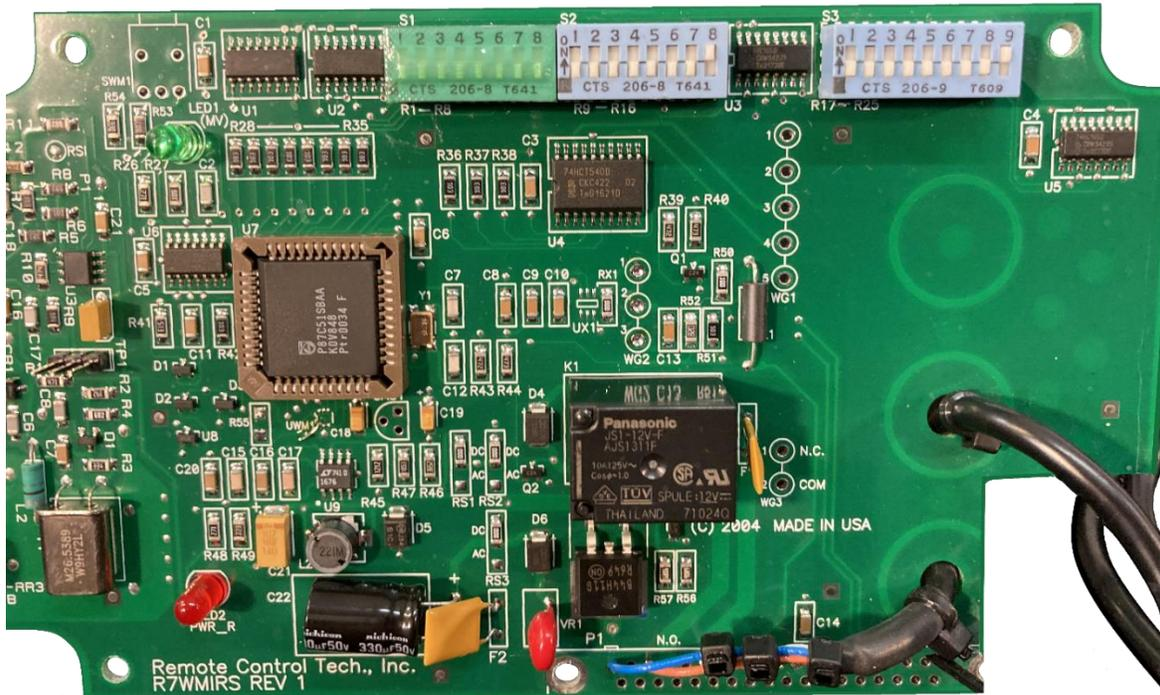
Per the photo above, this is the factory default setting: Group Code is set to “1” via the middle 8-Position DIP Switch & the Receiver Code is set to “1” via the right hand 9-Position DIP Switch.
