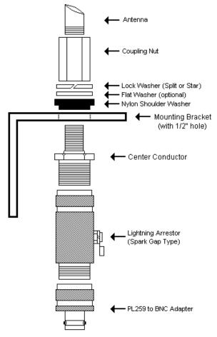
NOTE: Nylon Shoulder Washer lip MUST be seated inside Mounting Bracket hole for proper insulation!
