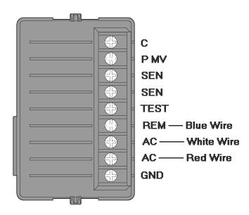
The Blue wire is connected to the terminal marked "REM" The White wire is connected to the terminal marked "AC" The Red wire is connected to the terminal marked "AC"
