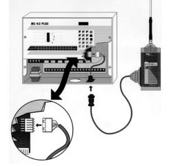
connect the DCI-2 and the universal receiver to the DCI-1. The first step is to connect the 37 PIN D-sub connector of the DCI-2 to the Universal receiver. Then connect the 9 PIN barrel connector to the DCI-1 installed in the controller.
