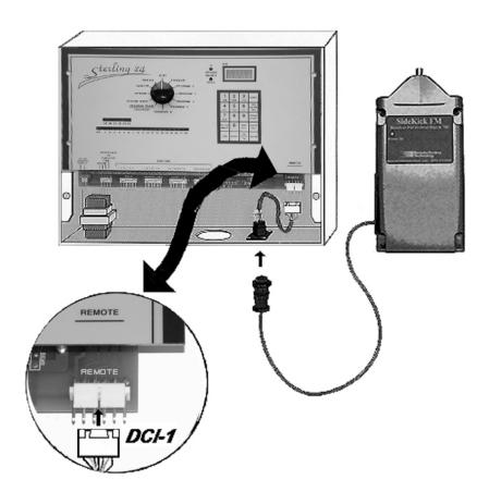
DCI-1 Cable and Sidekick Receiver installation (800) 275-8558 www.irrigationremotes.com
