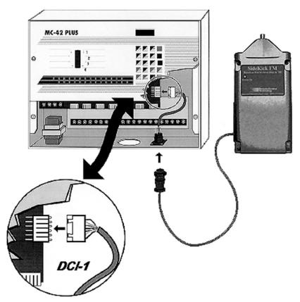
DCI-1 Cable and Sidekick Receiver installation
