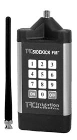
When not in use the transmitter reverts to a standby mode, which is designed for minimal power consumption to extend the life of the battery. Once any key has been pressed, power is automatically restored for ten seconds to allow commands to be sent to the receiver. The Transmitter is designed to operate using a 9 VDC Alkaline battery. **NOTE: Batteries such as general-purpose 9 VDC batteries will lower the performance of the transmitter.**
