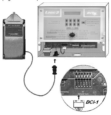
DCI-1 Cable and Sidekick Receiver installation
