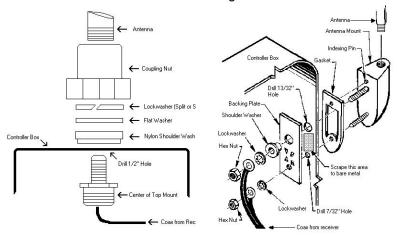
Top Mount Antenna Diagram Side Mount Antenna Diagram
